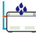
Figure 9. Fan coils in dehumidification mode.
