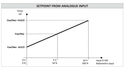
Correction calculation with ratiometric input (b20=1):
