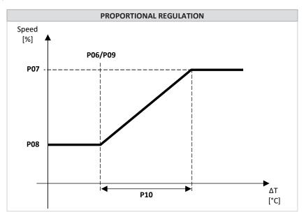
In practice, in cooling mode, if the temperature difference between the inlet and outlet is greater than P09 + P10, the circulator runs at maximum speed, but if the difference is less than P09 - 0.2°C, it runs at minimum speed; in the remaining cases, the pump modulates the speed proportionally. In heating mode, the same considerations apply, replacing parameter P06 with parameter P09. In sanitary production the circulator always runs at maximum speed.
