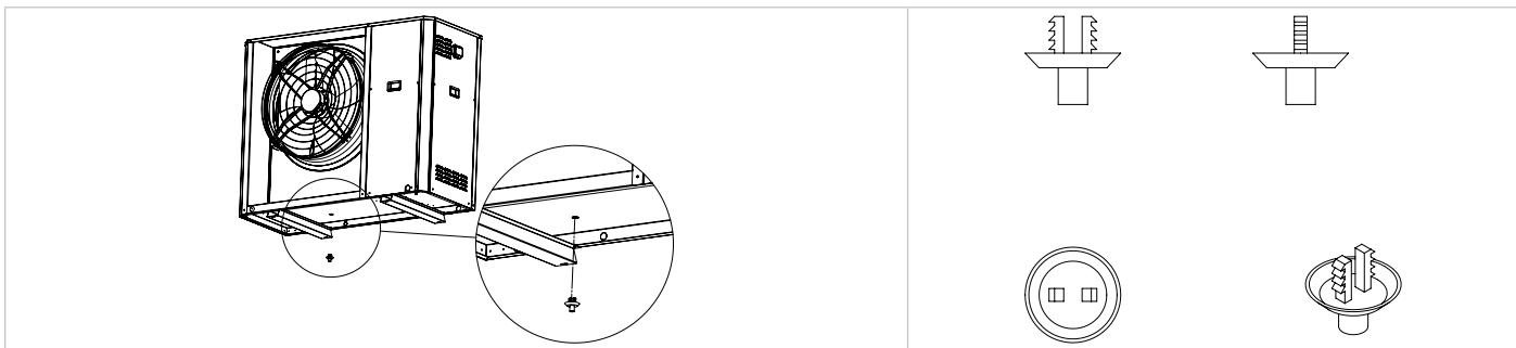
FOR HEAT PUMP UNITS, IN PARTICULARLY RIGID CLIMATES, THE INSTALLATION OF THE KA ACCESSORY IS RECOMMENDED, WHICH PREVENTS THE FORMATION OF ICE ON THE BASEMENT.
