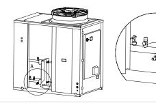
If the unit must be completely drained, first close the manual inlet and outlet shutters (not supplied) and then disconnect the pipes on the water inlet and outlet so that the liquid in the unit can drain (to make this operation easier, it is advisable to install two external drain cocks between the unit and the manual shutters on the water inlet and outlet).
